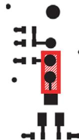
Jumper: Functionality activated -> Variation of voltage range with tuneable resistor between  $(2 \times V_{CC3}/3 - 0.5V = 1.7V)$  and  $(2 \times V_{CC3}/3 + 0.5V = 2.7V)$
