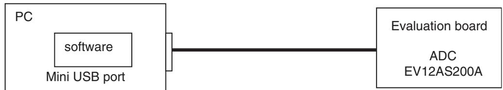
1. Use an mini USB port to send data to the ADC.
