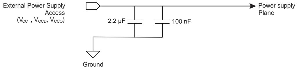
Note:  $V_{CCD}$  and  $V_{CCO}$  planes should be separated but the two power supplies can be reunited by a strap on the board.
