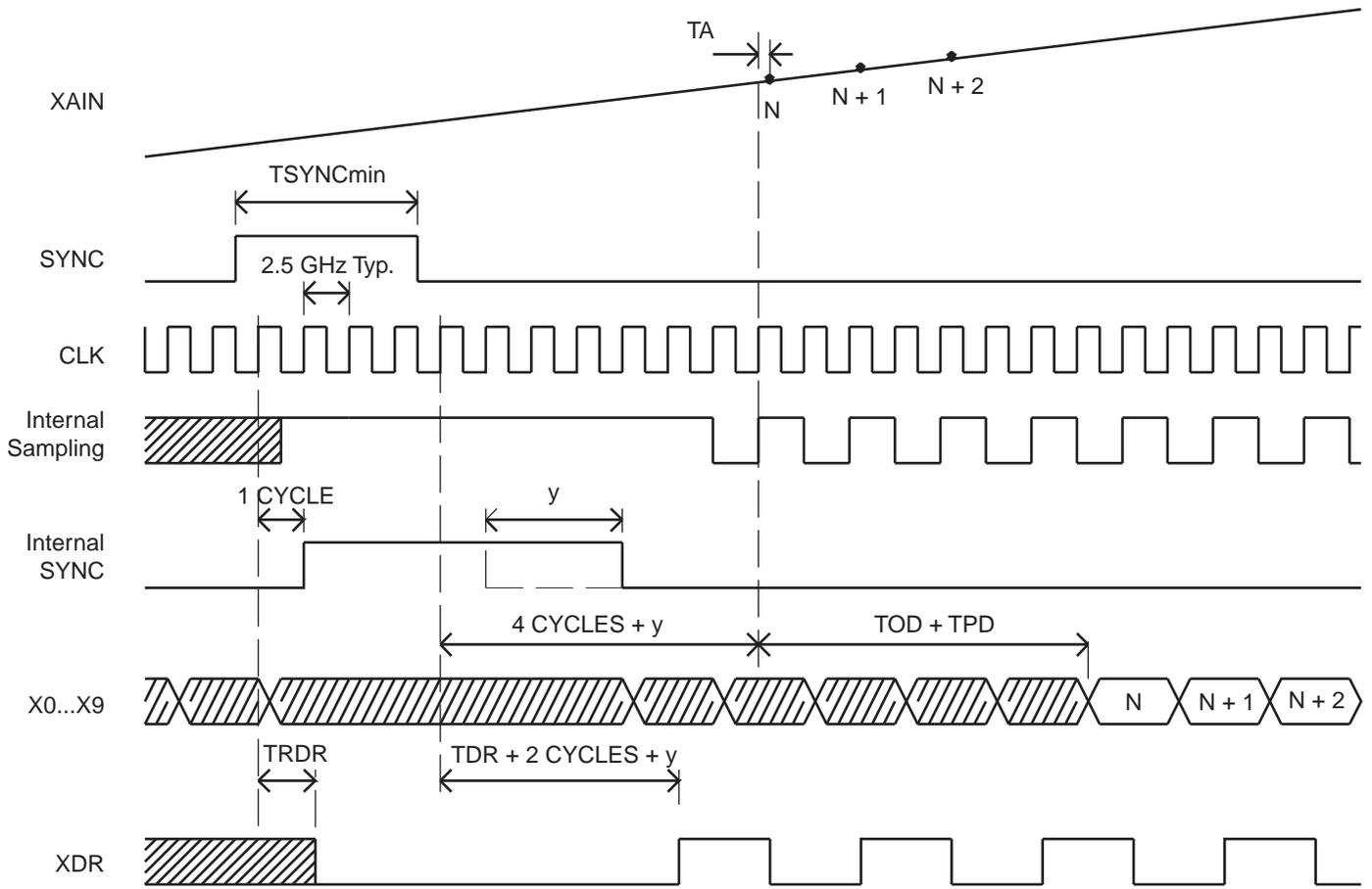
Figure 6-2. ADC SYNC Timing in Four-channel Mode, RM=1, SYNC Register y = 3 (Tunable 0 to 15 Cycles)
