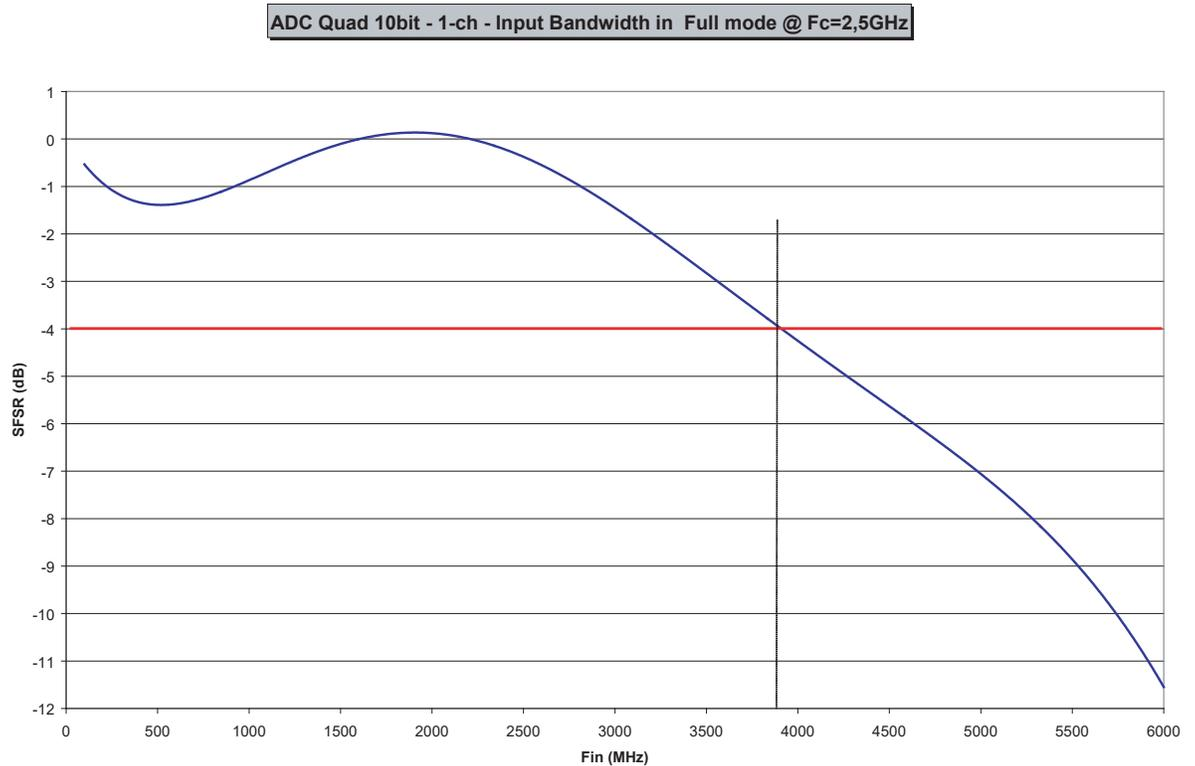
**Figure 4-2.** Full Power Input Bandwidth (-1 dBFS Input, 1-channel Mode,  $F_c = 2.5\text{GHz}$ , Nominal Bandwidth Setting)
