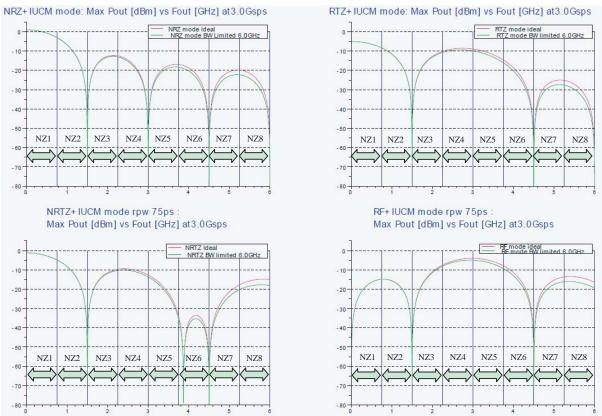
**Figure 5-9.** Max available Pout[dBm] at nominal gain vs Fout[GHz] in the four output modes at 2 GSps, combined with IUCM, over four nyquist zones, computed for  $T_{\tau} = 75$  ps
