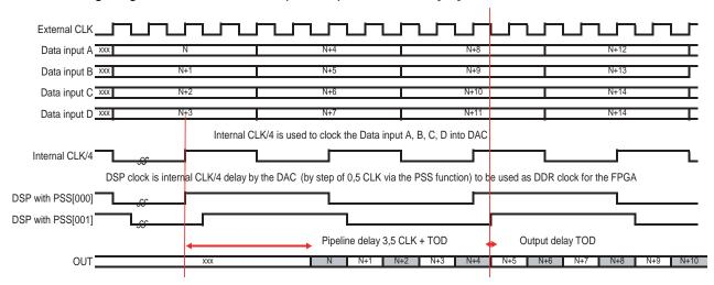
Figure 3-2. Timing Diagram for 2:1 MUX Principle of Operation OCDS[00]
