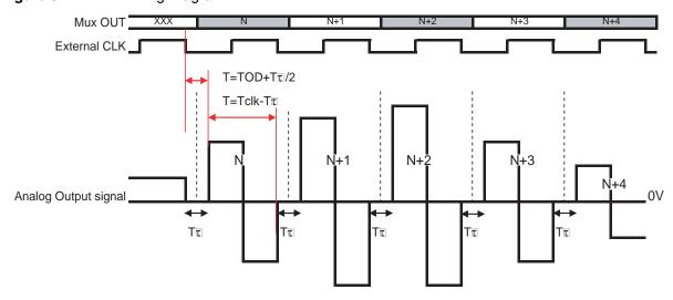
Note: The central transition is not hazardous but its elimination allows to push clock spur to 2.Fs  $T_{\tau}$  is independant of Fclock.
