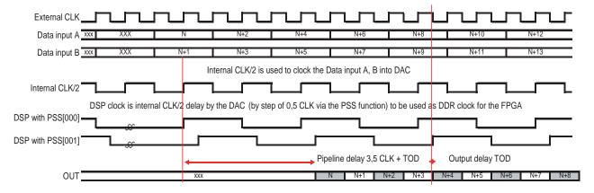
Figure 3-3. SYNC Timing Diagram
