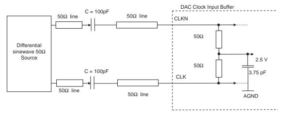
Note: The buffer is internally pre-polarized to 2.5V (buffer between V<sub>CCA5</sub> and AGND).
