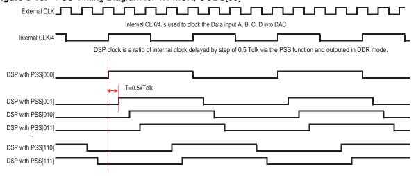
Figure 5-11. PSS Timing Diagram for 2:1 MUX, OCDS[00]
