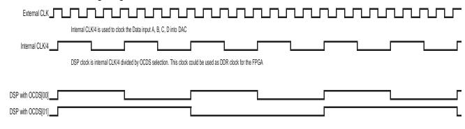
Figure 5-13. OCDS Timing Diagram for 2:1 MUX
