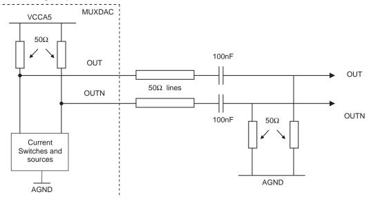
**Figure 7-2.** Analog Output Using a  $1/\sqrt{2}$  Balun
