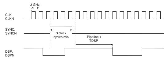
Figure 5-17. Reset Timing Diagram (2:1 MUX)
