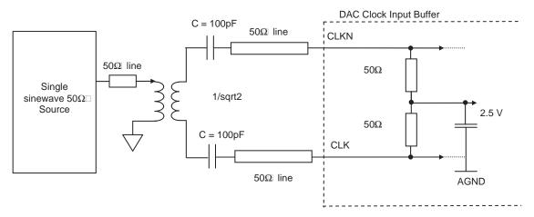
Note: The AC coupling capacitors should be chosen as broadband capacitors with a value depending on the application.
