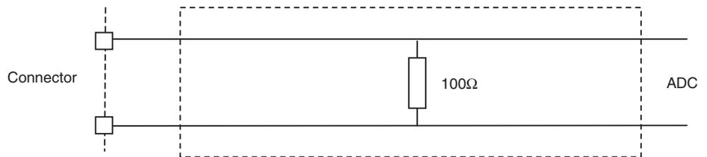
Double row 2.54 mm pitch connectors are used for the digital output data. The upper row is connected to the signal while the lower row is connected to Ground, as illustrated in Figure 2-4.
