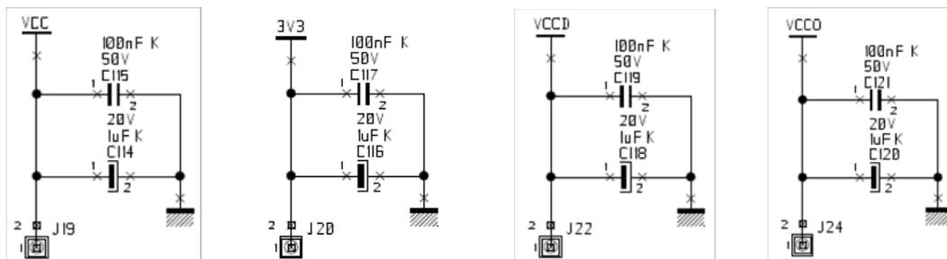
Figure 7-2. Power Supplies Decoupling (J = ± 5% Tolerance)
