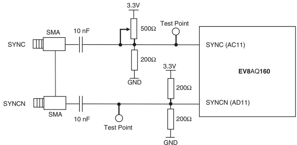
The resistors are used only for pull up and down of the SYNC signals. For reset, apply a pulse signal with a pulse generator via the SYNC SMA or apply directly a DC voltage (0.9V-1.3V) via the test points
