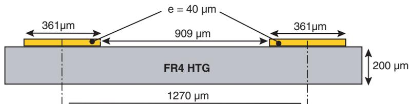
**Figure 2-6.** SYNC, SYNCN Inputs Implementation
