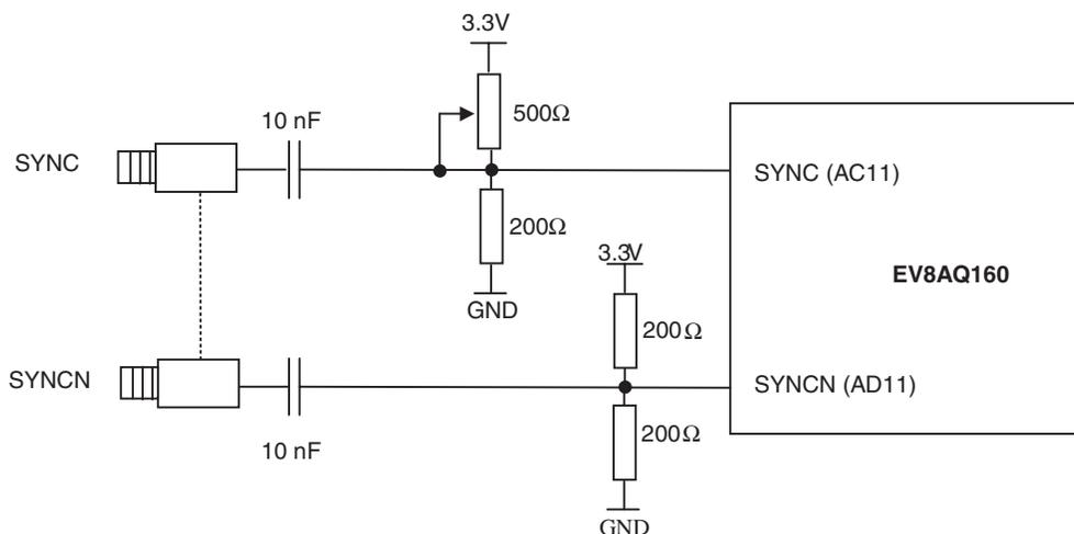
The resistors are used only for pull-up and pull-down of the SYNC signals. A push button is provided for the RSTN reset, as described in Figure 2-7 on page 2-9. This reset can also be generated through the AVR (via the User Interface).
