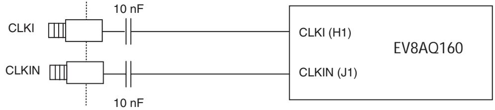
If used in single-ended mode, CLKIN should be terminated to ground via a 50Ω resistor. This is physically done by shorting the SMA on CLKIN with a 50Ω cap.
